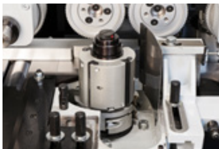
Axial adjustment range up to 75 mm
