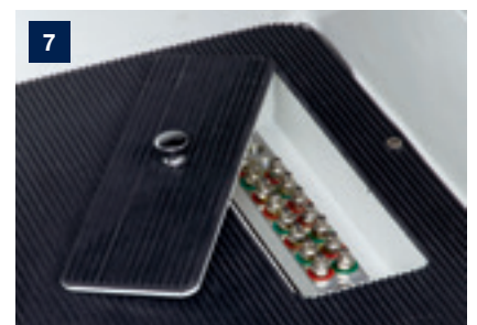
Accessible central lubrication at machine front
