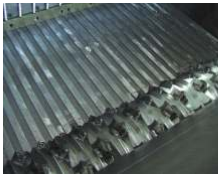
Serrated Ram for thin material
