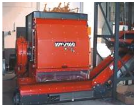
WL15 Shredder and conveyor belt with magnetic shut-off switch
