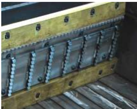
Pronged rail in the ram to avoid material spinning
