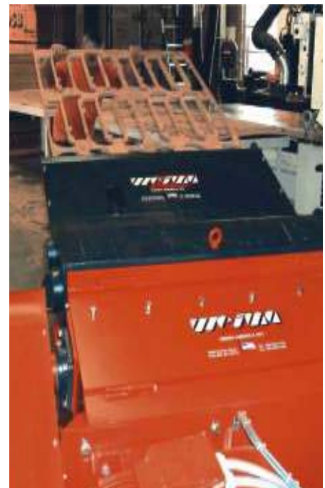
Beaver 1300 for skeleton grinding next to CNC Router
