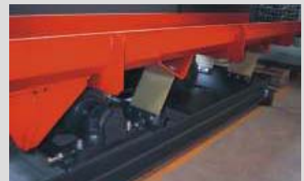
Modular vibrating conveyor system with integrated drive-train for easy installation
