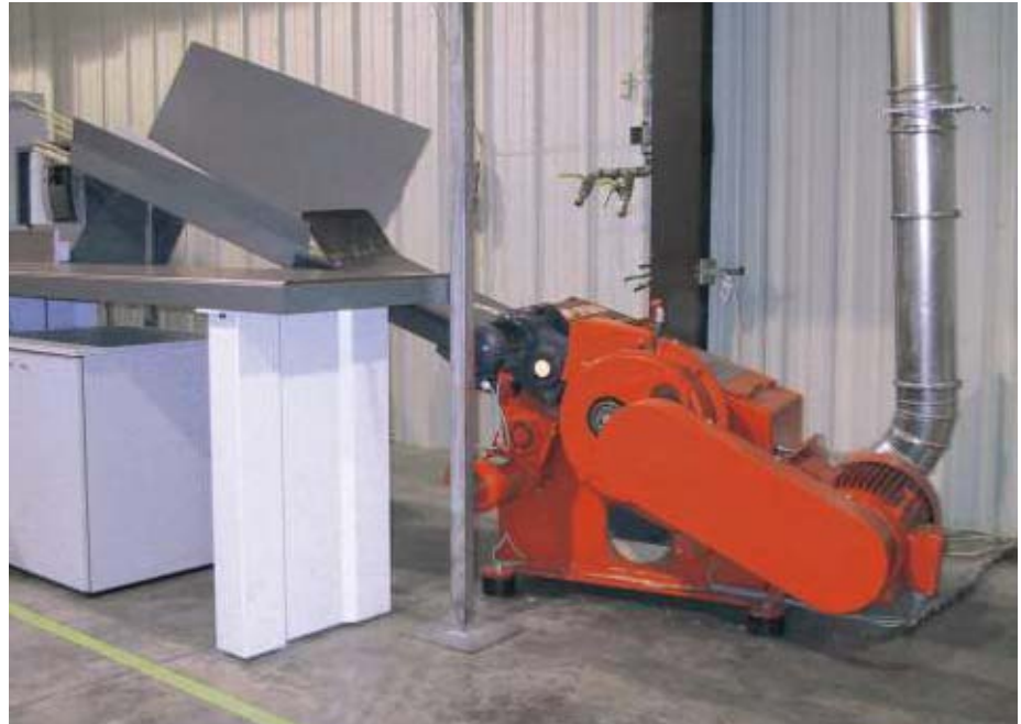
Beaver 600 in panel saw application with optional drop chute
