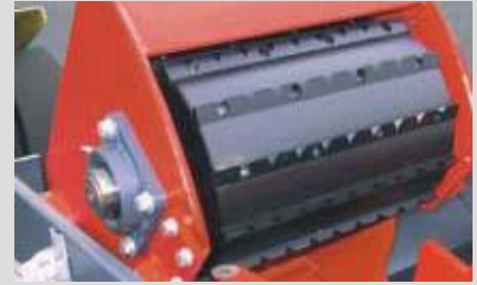
Pinch roller system with replaceable, aggressively shaped infeed bars
